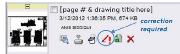
The city's E-Plan interface provides notes from each reviewer and indexed CD pages marked with a red pen icon to guide your architect's revisions. At the scale of individual drawing sheets, the element to be revised is surrounded by a red outlined 'revision cloud' and/or a small red note. Between the note comments –on code conflict, absent detail or supporting drawings, or missing elements– and drawing annotations, your design team should understand the issues at stake.
